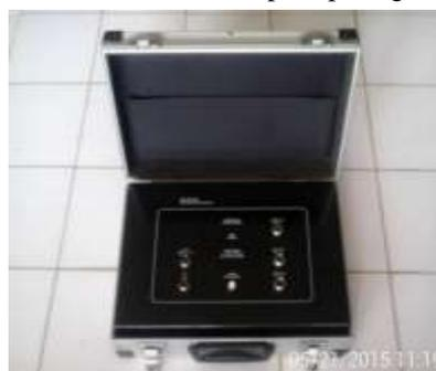
Gambar 2.3 Alat geolistrik multi channel
